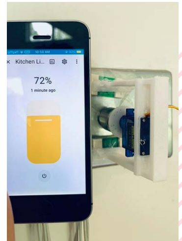
▲ An ingenious way of turning the dimmer switch using a servo and a sliding meter
