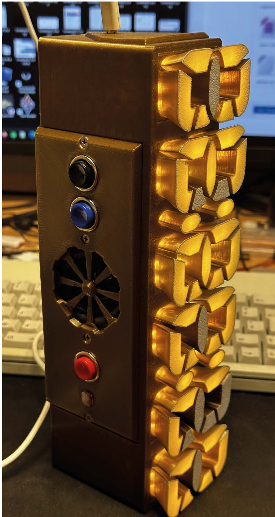
Right ♦ The whole thing is built into a 3D printed enclosure, complete with chunky buttons
