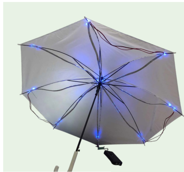
▲ Since all of the lights were connected in one long chain, Thomas only needed to use a single data pin on the Pico to control them all
