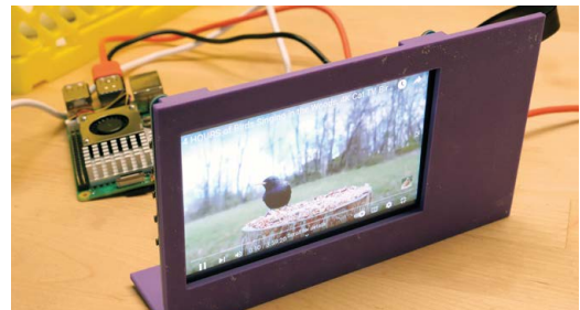
▲ Raspberry Pi Zero and an Elecrow touchscreen form the project's basis, all wrapped in a custom enclosure
