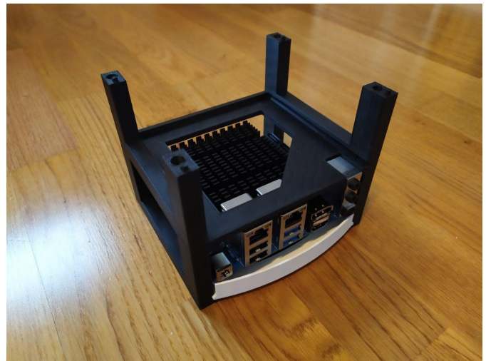
Figure 18 - The second mount print, where the alignment knobs work well, but the holes need to be cleaned of plastic for them to do their job properly
