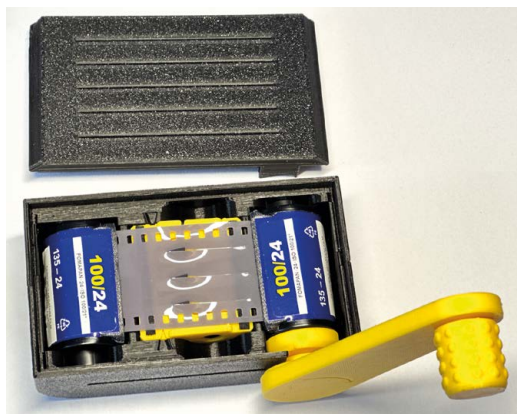
Figure 4 ♦ You can also get a slicing block that will cut a 16mm wide film strip to be used in other miniature cameras
