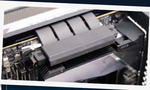
PCI-E riser cables are used to connect a graphics card to your motherboard's PCI-E slot in sandwich-style cases, or in cases with vertical graphics card arrangements
