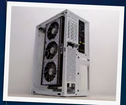
Even the largest graphics cards can fit inside mini-ITX cases, such as this GeForce RTX 3090 Ti installed in a Ssupd Meshlicious
