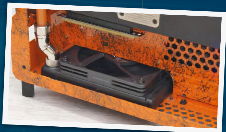
You can occasionally install slim fans and radiators in places that can't accommodate normal-sized models
