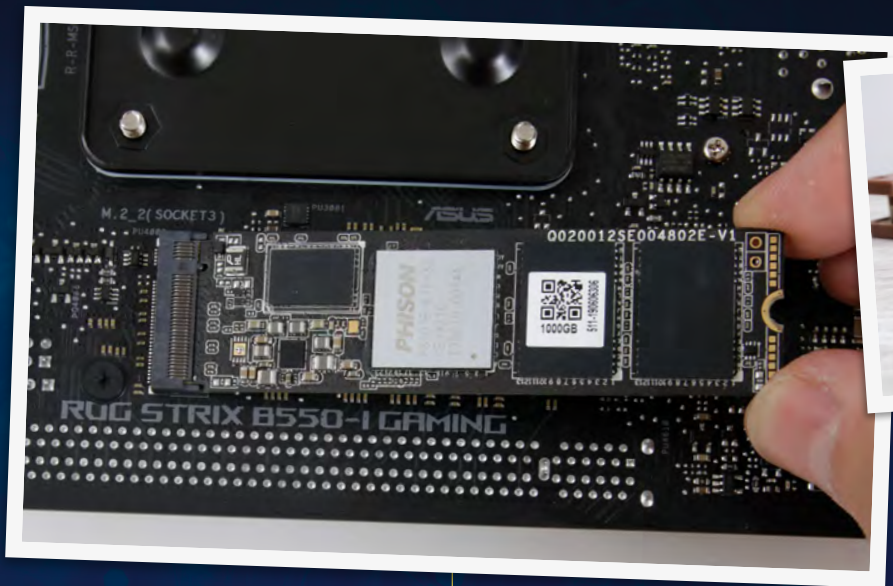
Using an M.2 SSD is a great way to cut cable numbers, as it connects straight to the motherboard, and 2TB models can now cost under £150
