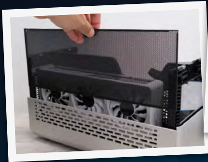
Make sure your CPU cooler and graphics card fans will be located near mesh panels
