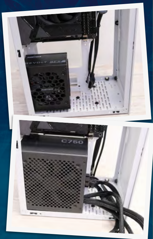
Using an SFX PSU (top) will free up a considerable amount of space compared to using an ATX PSU (bottom)
