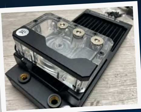
Small combined pump and reservoir units, such as EK's FLT 80, are ideal for water-cooling systems in mini-ITX cases
