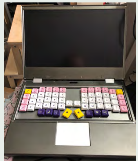
Jacqueline's customised Reform includes a new keyboard and a revised motherboard with USB Type-C charging
