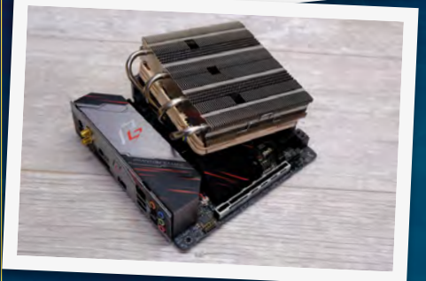
An example of the CPU cooler compatibility lottery is Noctua's NH-L12S, which fits fine on Gigabyte's X570i Aorus Pro WiFi (top), but doesn't stand a chance on ASRock's X570 Phantom Gaming ITX/TB3 (bottom)
