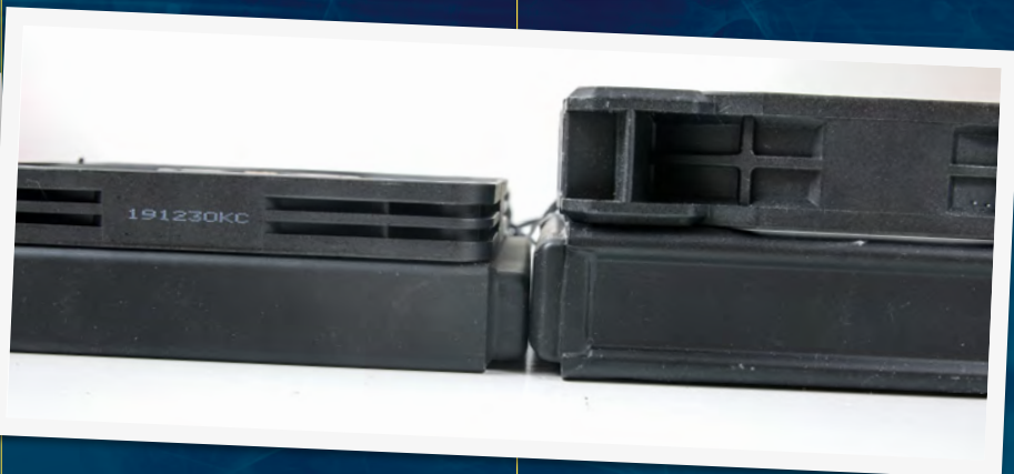
Using a slim radiator and slim fan shaves 2cm off the clearance compared with standard-height models
