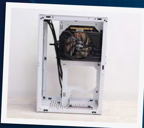
If you use a short graphics card, the Ssupd Meshlicious can house it horizontally instead of vertically, making room in the base for hard disks
