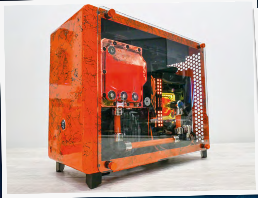
Small combined pump and reservoir units, such as EK's FLT 80, are ideal for water-cooling systems in mini-ITX cases
