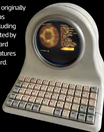
Jacqueline's customised Reform includes a new keyboard and a revised motherboard with USB Type-C charging
